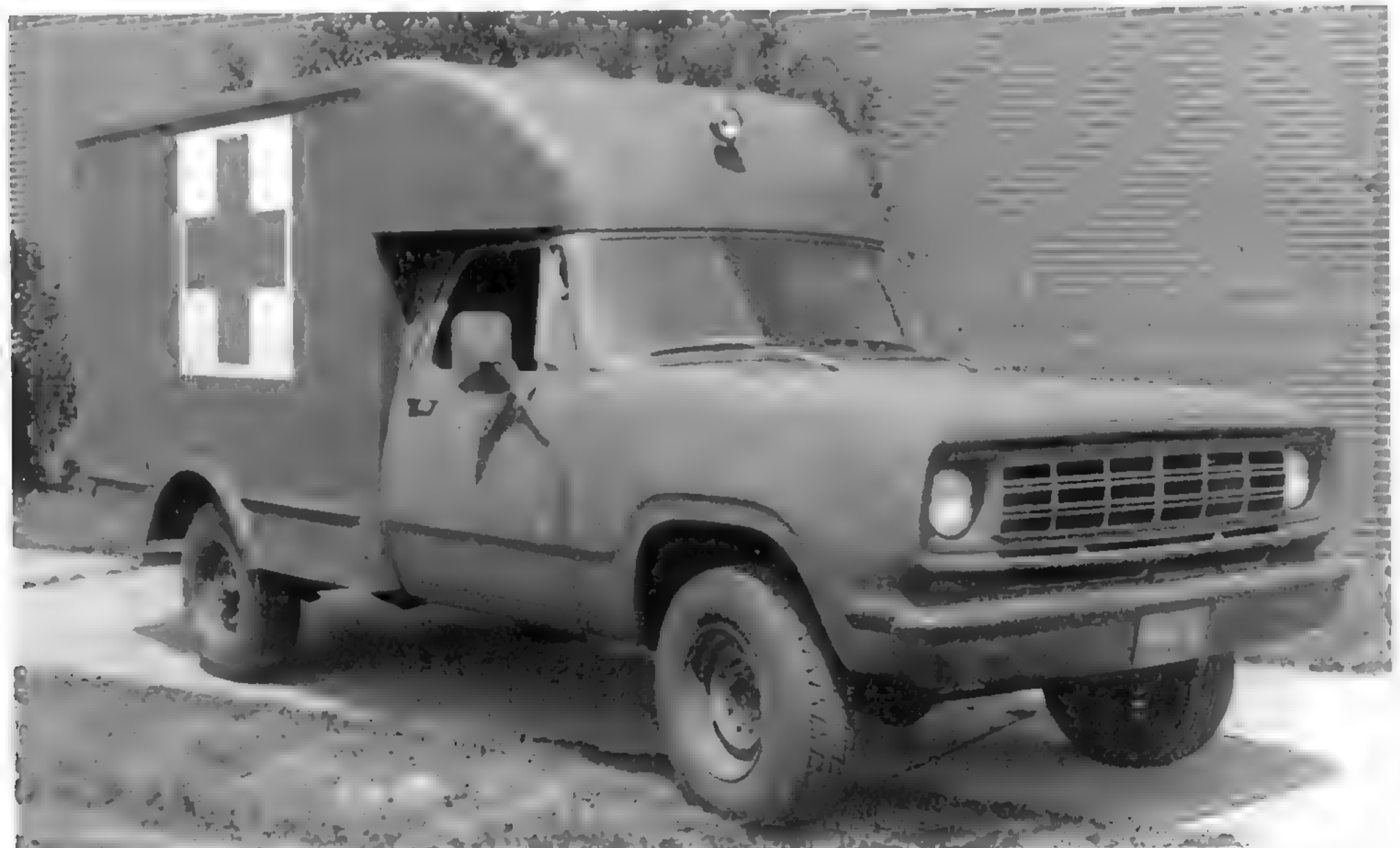
The M886 ambulance had an unmistakable profile. Some of these were adapted for use as communication vehicles. A spotlight was mounted on the front of the ambulance body. For any use other than ambulance, the red crosses would have been removed. (U.S. Army photo)
